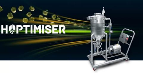
This brewing system has been specially designed to achieve rapid and complete contact during dry hopping to reach the pinnacle of hop flavour without developing undesirable hop characters.
