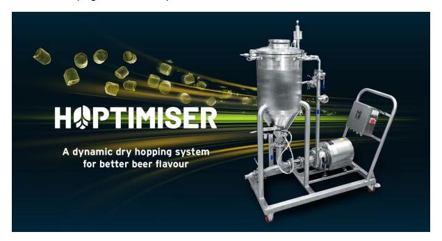
The system includes a pressurised container that feeds hop material into the beer stream before passing through a macerating pump. The resulting interaction with fine hop particles facilitates the uptake of key hop flavours while minimising astringency and hop burn.
